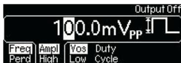
**NOTE** A momentary disruption in the output waveform may occur while changing amplitude. You can disable the voltage auto ranging function (refer to [Setting voltage auto ranging](#)) to prevent output disruption.
