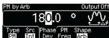
4. Press the soft key under **Src** to select between internal source (**Int**) and external source (**Ext**) for the modulating waveform ([Figure 5-13](#)). If internal source is selected:
