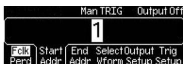
5. Press the soft key under **End / Addr** to specify an end point for the pattern output ([Figure 5-23](#)). Use the navigation wheel with the cursor keys to change the value, and then press another soft key to finish the entry and exit. Or use the numeric keypad to enter a desired value and then press the soft key under **Enter** to finish the entry, or the soft key under **Cancel** to cancel the changes.
