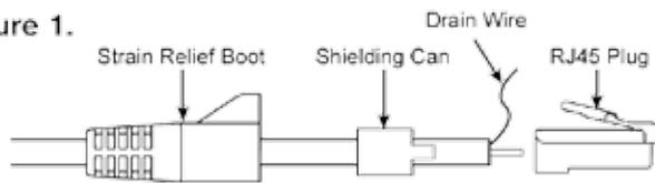
Prepare cable as you would for UTP assemblies. Place the boot onto the cable, followed by the metal can, as shown above.
