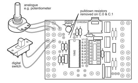
The connections marked C.3 and C.4 should not generally be used with the PICAXE system. These are used by the PICAXE chip as the 'serial in' and 'serial out' PC download connection.
