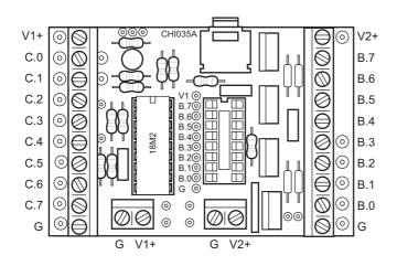
Note that when using terminal blocks it is necessary to 'share' the V2+ connector with all output pins and to 'share' the V1+ connector with all inputs. Remember that with the FET output buffer the output devices are connected between V2+ and the output (NOT output to 0V). Like wise the inputs are connected between V1+ and the input.
