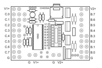
To use the board with an older (now discontinued) 18/18A/18M/18X PICAXE part an extra 1k resistor \***MUST**\* be soldered to the board in the 'RST' resistor position. If desired an optional reset switch (part SEN030) may also be fitted in position 'S1'. Note that the current release PICAXE-18M2 does not have a reset pin, so does not require the RST resistor or the reset switch to be fitted.
