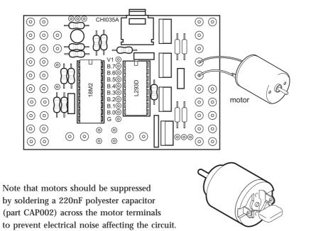
Outputs B.4 & B.5 control one motor, outputs B.6 and B.7 control the other motor.
