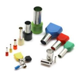
TRU Components wire end ferrules guarantee optimal crimp connections in conjunction with fitting crimping tools. This product series includes wire end ferrules with plastic collars as well as double wire end ferrules in all colors based on the DIN color code. The ferrules are especially suitable for
