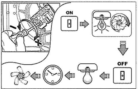
Adjust the trimmer (screw) illustrated in the figure to increase or decrease the delay in turning off the device (from 3 to 25 minutes).
