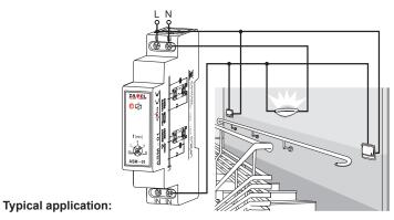
The staircase lighting time delay switch ASM-01 operating the staircase lighting works in 3-wire installation. Monostable pushbutton (equipped with illumination) can be connected parallely.
