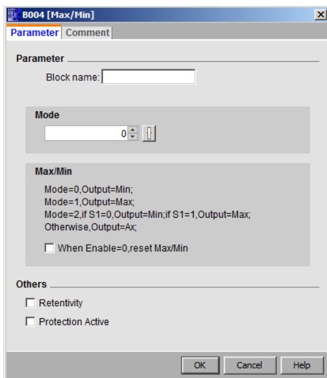
If you select the check box "when Enable = 0, reset Max/Min":
