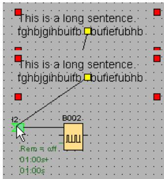
A linked comment moves consistently with the figure to which it is attached. You can adjust the relative position of the comment to the figure, as you do a block comment.
