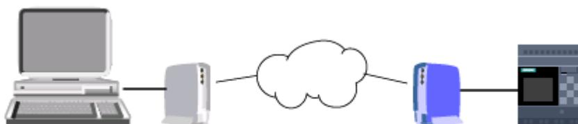
Select the **Tools** → **Connect Modem** menu command to start the process of configuring modems connected to your PC with LOGO!Soft Comfort. The LOGO! Base Module at the remote side is also connected with a modem and ready for network connection. LOGO!Soft Comfort displays a Modem Information dialog that provides an overview of the configuration process.
