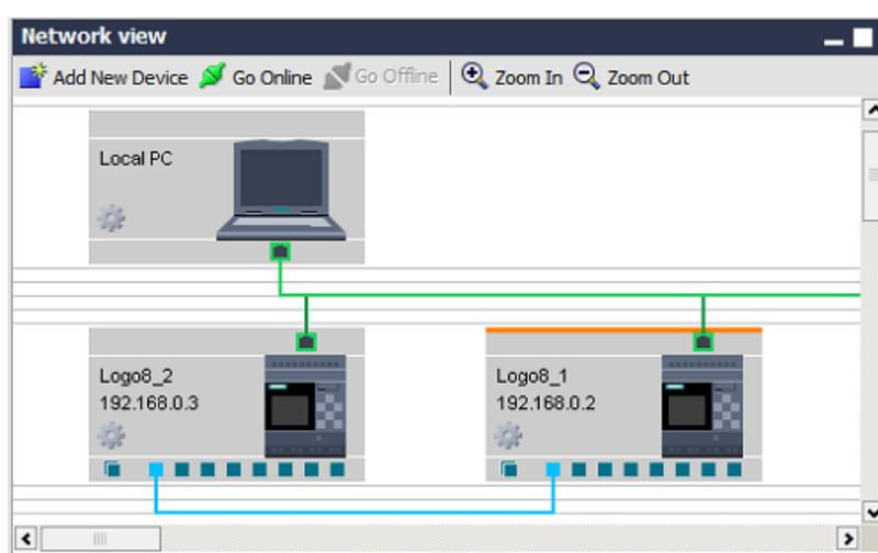
If you use the LOGO! Base Module as a dynamic server, LOGO!Soft Comfort supports to use drag-and-drop to create dynamic connections from the LOGO! Base Module to multiple client devices. LOGO!Soft Comfort automatically identifies the server and client according to your operations.
