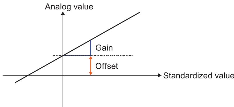
The straight line in the graphic describes which standardized value is being converted into which analog value. Gain corresponds to the slope of the straight line and offset to the movement of the zero point of the straight line on the y-axis.
