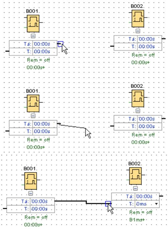
2. You can cut and rejoin the reference line. For information on cutting the reference line, see [Cut/Join \(Page 39\)](#).
