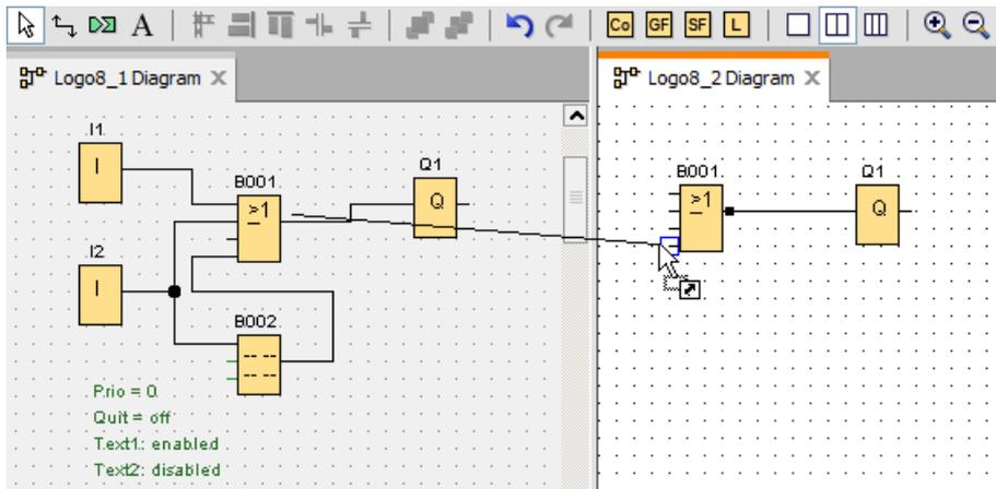
When you connect two function blocks in two separate circuit diagrams, LOGO!Soft Comfort creates a pair of network function blocks, including the Ethernet connection and data transfer mechanism. The green color indicates that the LOGO! device of the two circuits are connected in LOGO!Soft Comfort. The network function block turns to red if its LOGO! device loses the connection to the other LOGO! device in LOGO!Soft Comfort.
