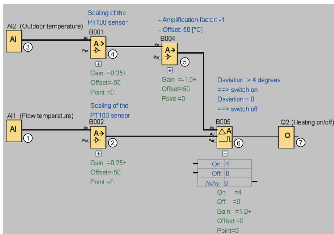
① A PT100 sensor is connected to AI1 which measures the flow temperature.
