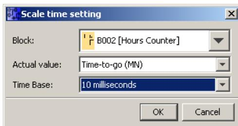
With this dialog, you can configure the scale time base for a function block value. You select a function block, an actual value and a time base, and click "OK" to confirm your settings.
