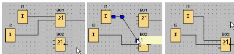
By keeping this block replacement order, you can maintain your connecting lines. If you first delete the old block, you also delete its connections, which means you have to recreate all connections.
