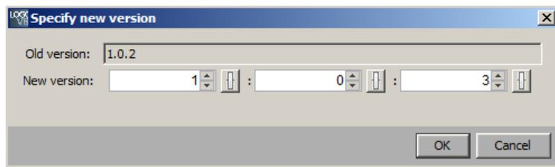
The new version must be an increment from the previous value. For example, in the example shown above, version 1.0.3 or 0.254.3 would be invalid.
