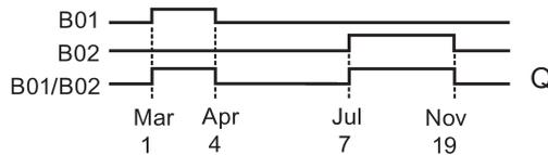
Place two yearly timer switch SFBs on your programming interface. Configure the On Time for the first yearly timer to 03.01 and the Off Time to 04.04. Configure the On Time for the second yearly timer to 07.07 and the Off Time to 11.19.
