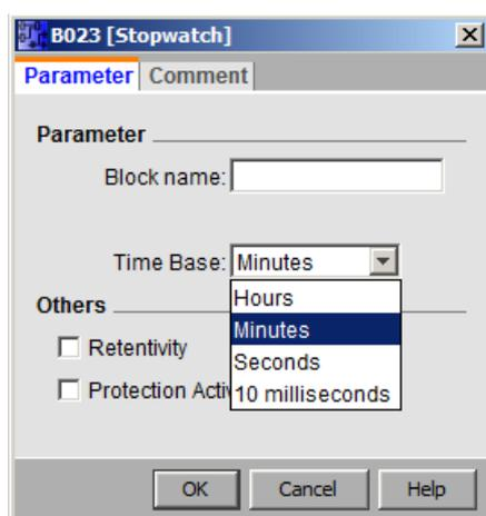
The time base for the elapsed time can be in hours, minutes, seconds, or 1/100ths of seconds (units of 10 milliseconds). The smallest time base, and therefore the resolution, is 10 milliseconds, or 1/100ths of seconds.
