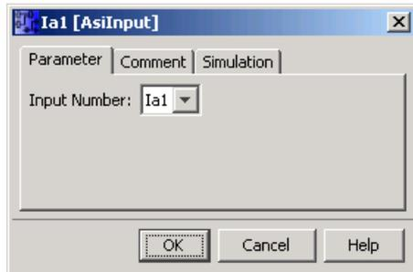
AS-Interface inputs are named Ia. The block number of an AS-Interface input is determined by the hardware structure.
