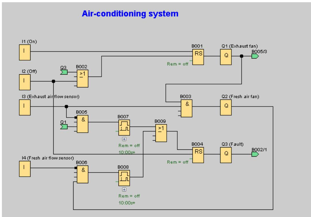
You can invert output Q3 to use output messages at Q4. Relay Q4 only drops out if main power is lost or if there is a fault in the system. The output can then be used for a remote message.
