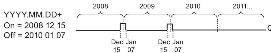
**Example 8: Monthly selected, On Time = 2008.\*\*.01, Off Time = 2010.\*\*.05.** Starting in 2008, on the first day of each month the timer output switches on and switches off on the fifth day of the month. The timer continues in this pattern through the last month of 2010.
