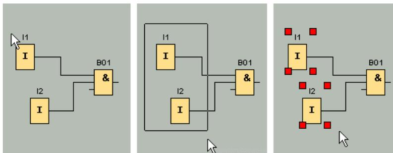
In addition to the selection of single objects by a simple mouse click or highlighting object groups by "capturing", there is a further selection option: Under "optional selection", mark the objects one after the other by holding down the [Ctrl] key while you select the objects. To remove an object from the selection, hold down the [Ctrl] key and click a selected object once again.
