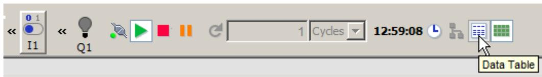
In the Data Table, you can enter VM addresses and choose the corresponding data types. LOGO!Soft Comfort displays the current values for the VM addresses that you provide. You can add new rows by right-clicking an existing row, or pressing the Enter key on the last cell of an existing row. You can enter new values in the New Value column for an existing VM address.
