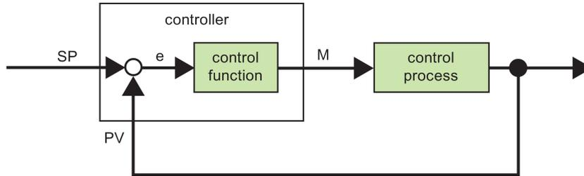
The comparing element and the controller function describe the conduct of the controller. The following describes the most important types of controller. A controller step response tells us a lot about its conduct. The step response describes how a controller reacts to the erratic change in the process value.
