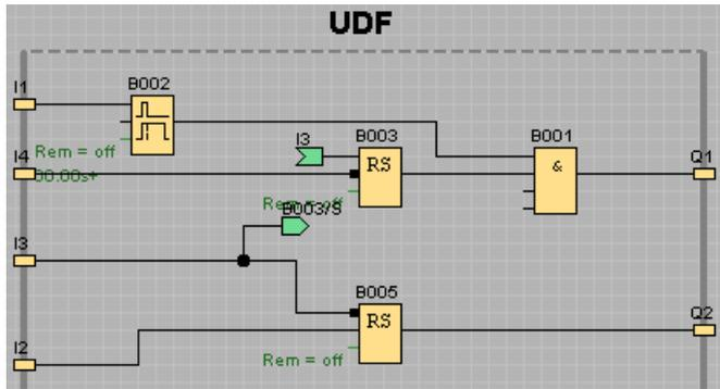
Note that UDF blocks do not support inputs, outputs, analog inputs, analog outputs, M8, M25, M26, M27, shift registers, the data log or message text function blocks.
