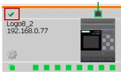
If the configured device is inaccessible, LOGO!Soft Comfort shows a question mark in the top-left corner of the device image.
