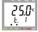
**No temperature sensor: manual input of temperature of buffer 2**
