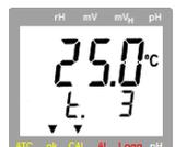
**No temperature sensor: manual input of temperature of buffer 3**
