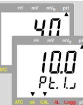
\*1) Place electrode and temperature probe (if any) in the third buffer solution (e.g. for standard series this is: pH 10.0) and stir gently.
