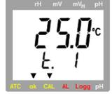
**No temperature sensor: manual input of temperature of buffer 1**
