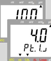
\*1) Place electrode and temperature probe (if any) in the second buffer solution (e.g. for standard series this is: pH 4.0 or pH 10.0) and stir gently.
