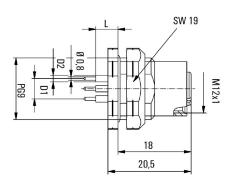
L(board-to-board distance) = 5,5mm D1 = 5,0 mm D2 = 1,6 mm
