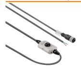
Motion detector for the WIL-LED luminaire with screw connection, 3m supply cable and M12 cable for connection to the WIL lamp. Switching time adjustable.
