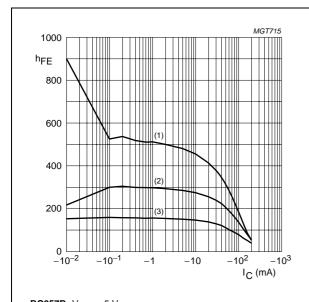
BC857B;  $V_{CE} = -5 \text{ V}.$
