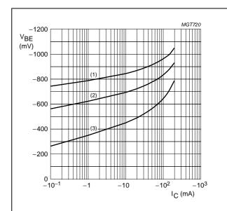
**BC857C**;  $V_{CE} = -5 \text{ V}.$
