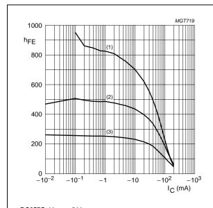
**BC857C;**  $V_{CE} = -5 \text{ V}.$
