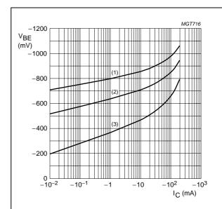
**BC857B**;  $V_{CE} = -5 \text{ V}.$
