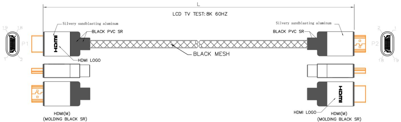
NOTE: E314459 况 AWM 20276 80°C 30V VW-1 HIGH SPEED HDMI® CABLE WITH ETHERNET
