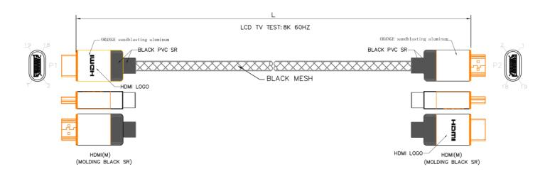
NOTE: E314459  $\pm$  AWM 20276 80  $\pm$  30V VW-1 HIGH SPEED HDMI CABLE WITH ETHERNET
