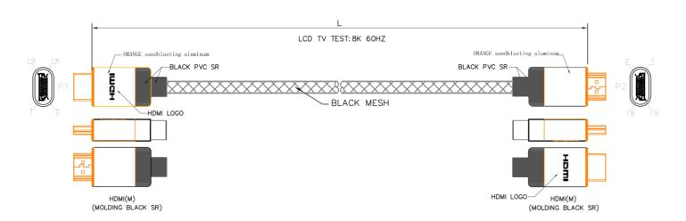
NOTE: E314459  $\,\%$  AWM 20276 80  $\,\%$  30V VW-1 HIGH SPEED HDMI  $^{\circ}$  CABLE WITH ETHERNET
