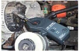
For this final example, alternator charging current and voltage was measured using the meter function in PicoScope. The current clamp needs to be switched on and facing the correct way. There is an arrow pointing to the battery positive (+) on one side and an arrow pointing to the battery negative (-) on the other side. Incorrect connection will lead to the incorrect polarity of the reading, in this case the alternator is generating current and we would expect to see a positive reading.
