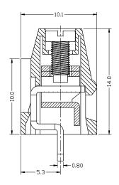
Measurements are in mm unless stated otherwise. Tolerance: ±0.2
