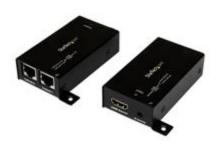
The ST121SHD30 HDMI® over CAT5e/CAT6 Video Extender kit lets you extend HDMI audio/video and an IR remote control signal by up to 100 feet (30 Meters) over dual Cat5e or Cat6 cable. For added versatility this HDMI extender kit is powered via the HDMI bus, and does not require any additional power adapter.
