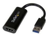
The USB32HDES Slim USB 3.0 to HDMI Adapter turns a USB 3.0 port into an HDMI output with 1920x1200/1080p video support. The adapter minimizes clutter with a slim design that seamlessly blends with your video cable - an ideal space-saving solution for multi-monitor applications on Ultrabook™, laptop, or desktop computers.
