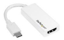
This USB-C™ to HDMI® adapter lets you output HDMI video and audio from a USB Type-C™ device such as a MacBook or Chromebook™ laptop. This adapter works with USB-C devices that pass a DisplayPort video signal. It's also compatible with Thunderbolt™ 3 ports.
