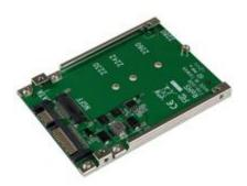
Vastly increase system performance by adding the speed of an M.2 SSD (Next Generation Form Factor) in any 2.5" SATA application, with the SAT32M225 M.2 SSD to SATA adapter.
