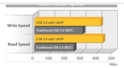
At the same peak in testing UASP also shows an 80% reduction in required processor resources.
