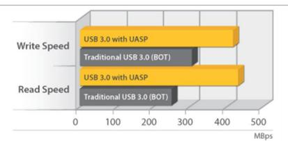
At the same peak in testing UASP also shows an 80% reduction in required processor resources.
