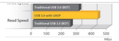
At the same peak in testing UASP also shows an 80% reduction in required processor resources.
