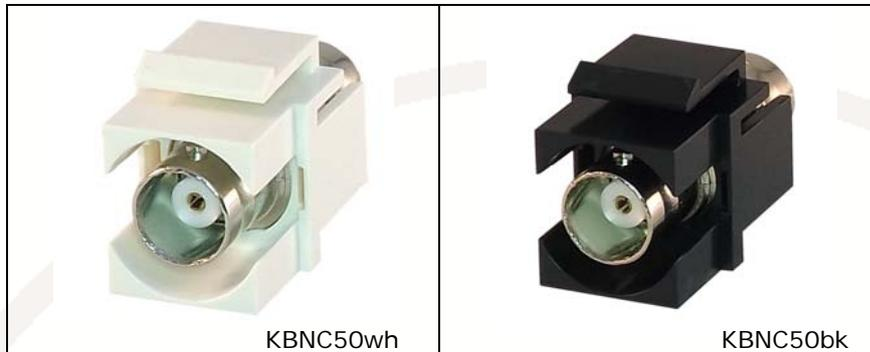
**The 50Ω BNC keystone jack is designed to support CCTV and NTSC analog video signals, as well as any application requiring 50Ω BNC connectors. It is designed to snap into any standard sized keystone outlets and patch panels.**
