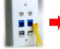
Simply pull out the removal tool to remove the PortBlocker.
