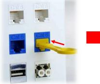
Ensure removal tool is straight i.e. while inserting tool make sure the arrow sign of the tool is facing position A
