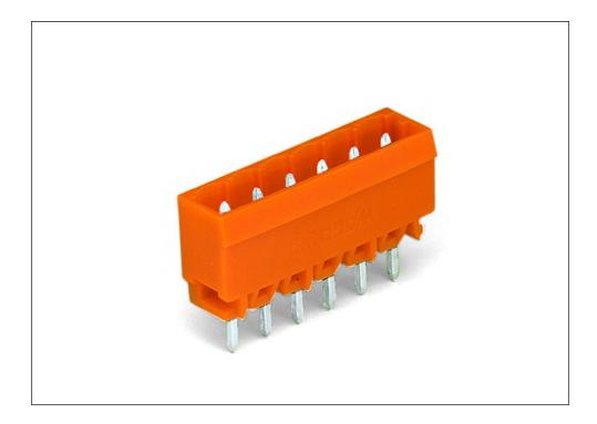
Printview: Male connector; with straight solder pins; 2-pole; Pin spacing  $5.08 \ \text{mm} \ / \ 0.2 \ \text{in}$ ; Vertical PCB mounting; with closed end - Item No.: 231-332/001-000
