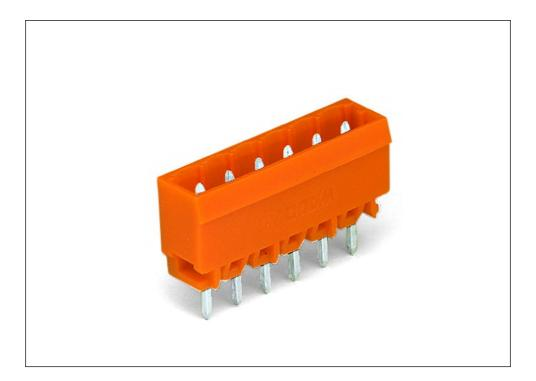
Printview: Male connector; with straight solder pins; 6-pole; Pin spacing  $5.08 \, \text{mm} / 0.2 \, \text{in}$ ; Vertical PCB mounting; with closed end - Item No.: 231-336/001-000
