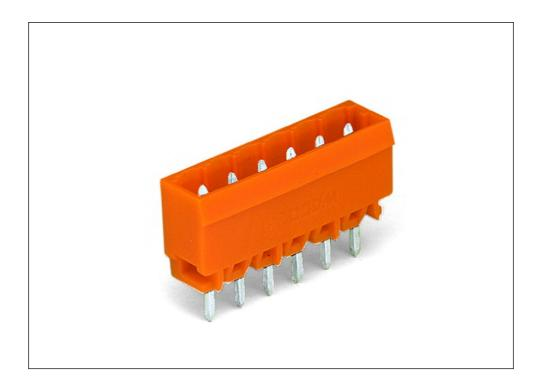
Printview: Male connector; with straight solder pins; 10-pole; Pin spacing  $5.08 \, \text{mm} / 0.2 \, \text{in}$ ; Vertical PCB mounting; with closed end - Item No.: 231-340/001-000
