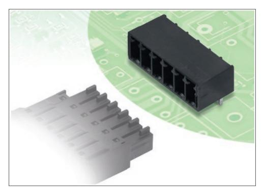
Printview: Male header (for PCBs); Straight solder pin 0.8 x 0.8 mm; 3-pole; Pin spacing 3.5 mm / 0.138 in; Vertical PCB mounting; with closed end - Item No.: 714-133
