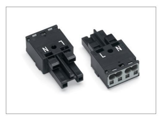
Printview: Socket; without strain relief housing; 2-pole; 100% protected against mismating; 2-conductor connection; Pin spacing 10 mm / 0.394 in - Item No.: 770-1102
