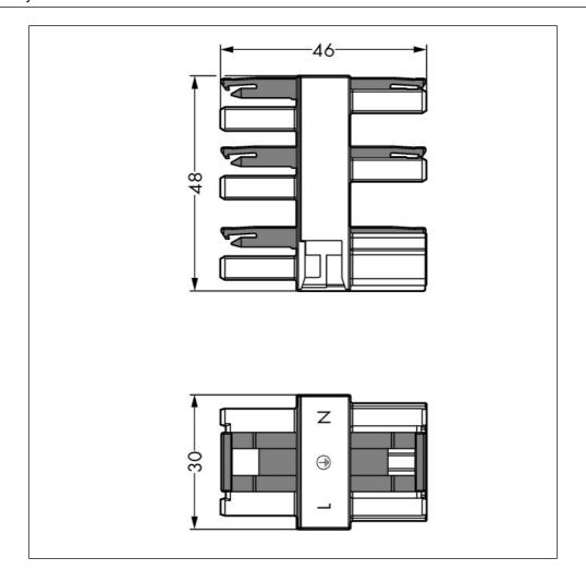
Printview: Distribution connector; 1 x plug / 5 x socket; 3-pole; 100% protected against mismating;
