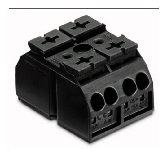
Printview: 4-conductor chassis-mount terminal strip; for mounting via M3 screw and nut or self-tapping screw 2.9 mm Ø from top; plain; with 2x pin; 2-pole - Item No.: 862-552
