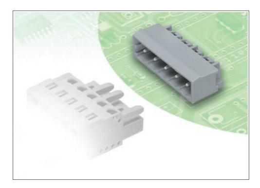
Printview: Male connector; with angled solder pins; 8-pole; Pin spacing 5.08 mm / 0.2 in; Horizontal PCB mounting; with closed end - Item No.: 231-538/001-000
