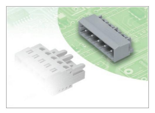
Printview: Male connector; with angled solder pins; 12-pole; Pin spacing 5.08 mm / 0.2 in; Horizontal PCB mounting; with closed end - Item No.: 231-542/001-000
