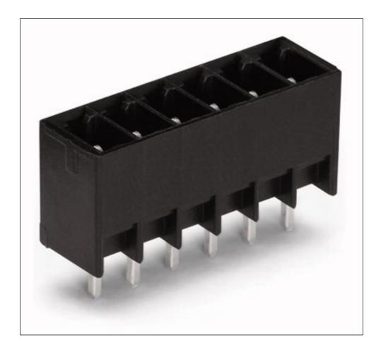
Printview: Male header (for PCBs); Straight solder pin  $0.8 \times 0.8$  mm; 6-pole; Pin spacing 3.5 mm / 0.138 in; Vertical PCB mounting; with closed end - Item No.: 714-136
