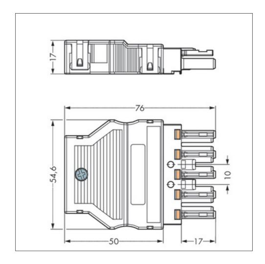
Printview: Socket; with strain relief housing; 5-pole; Pin spacing 10 mm / 0.394 in; 100% protected against mismating; Cable diameter 9 - 13 mm - Item No.: 770-105
