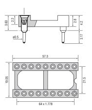
High density DIL socket for devices featuring 0.07" (1.778mm) lead spacing.
