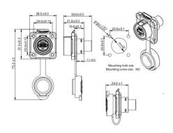
Cable O.D. range:  $\emptyset 3.0 \sim \emptyset 7.0 \text{ mm}$ Temperature Range:  $-25^{\circ}\text{C}$  to  $+85^{\circ}\text{C}$
