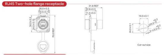
Cable O.D. range: Ø3.0~Ø7.0 mm Temperature Range: -25°C to +85°C
