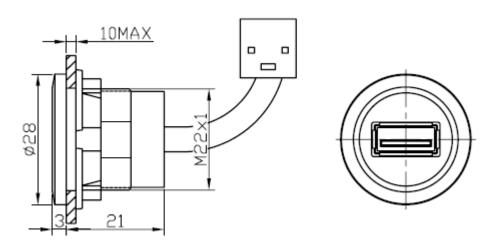
10MAX: means the panel thickness, the max thickness for the panel no more than 10mm.
