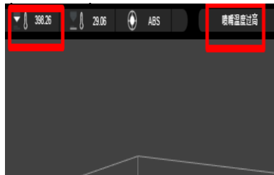
Printing stops and reports nozzle high temperature error
