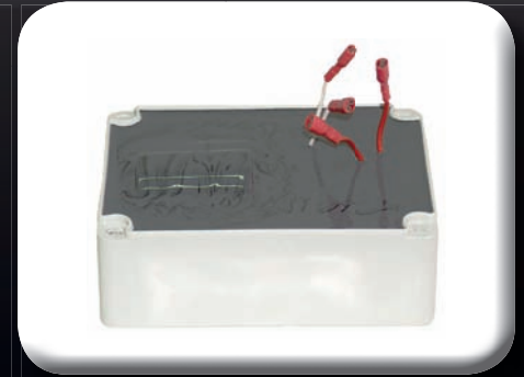
Insulation of components by immersion in magic Rubber
