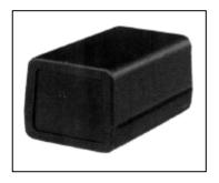
A two-part ABS case with black textured finish and removable ABS front panel. Ideal for use as a transformer or power supply case or for housing a printed circuit board. Six bosses, suitable for self-tapping screws, are molded into the bottom part of the case for mounting PCBs or a chassis plate. The two halves of the case are held together by four self-tapping screws, which are supplied.
