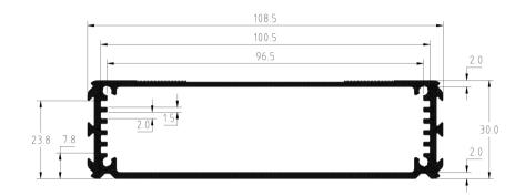
Length Tolerance: Nominal length -0mm/+1mm e.g. EBS 80 is not shorter than 80mm and not longer than 81mm.
