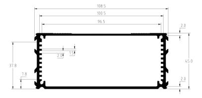
**Length Tolerance:** Nominal length -0mm/+1mm e.g. extrusion ECS 80 is cut not shorter than 80mm and not longer than 81mm.
