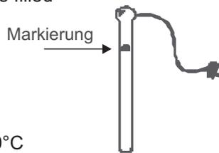
4. Connect the power cord of the glass heater to mains voltage (AC 230V/50-60Hz). Turning the adjustment knob in plus-direction (cw) increases the temperature, the temperature is reduced by turning into the minus direction (ccw)
