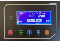
returns to the bottom of the display and STOP to the top and you can restart heating by pressing the **RUN** key.
