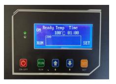
If you press SET instead of RUN, then READY (pre-heat-phase) will be highlighted. Use the arrow keys to change the text to HEAT, WELD, HOLD or COOL. Stay on READY and press **SET**. The marking jumps to **TEMP** (temperature) and you can adjust the temperature between 70 and 130°C with the arrow keys. Another press on SET and you can change the time between 00:00 and 99:99 (minutes: seconds).
