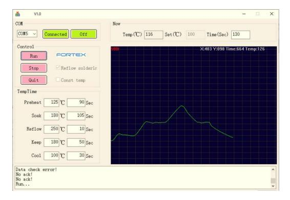
Next in the software tick the box next to "Reflow Soldering". Temperature and Time values can now be entered to set each section for the desired reflow parameters.
