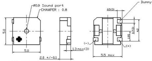
Unit : mm General Tolerance : +/- 0.2(if not specified) Housing material : LCP
