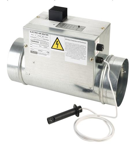
Similar to other NEATAFAN in-built thyristor controllers the TC3 has a temperature set-point control on the front facia and Indicator lamps to show the status. The heater units come with a pre-wired high temperature manual reset cut-out, a pre-wired duct mount combined DTFS airflow proving and temperature sensor on a 1.8 metre fixed lead. This should be mounted a minimum of 1M after the heater in the supply air duct.
