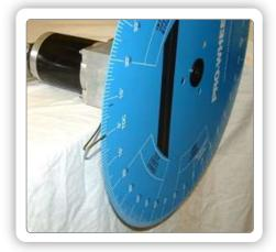
The gearhead is tested for backlash by locking the motor in place. A load of 200 ounce-inches is applied in both clockwise and counterclockwise directions. The total deflection is +/- 1.2 degrees. This figure may increase somewhat with higher loads and chain wear, but replacement chains are available.
