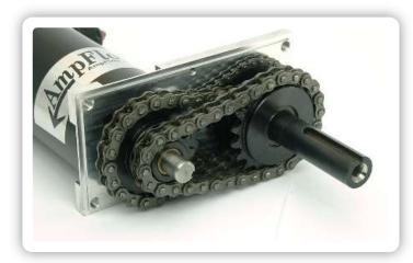
The output shaft is 3/4-inch diameter and 2.2 inches long. It has a 1/4-inch keyway and a 5/16-24 tapped hole. The shaft and the large final sprocket are made from a single piece of steel to maximize strength. If something other than the 1/4-inch key is required, step key stock is available.
