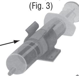
20mm Syringes can also be held firmly in place but because they are of a slightly smaller diameter they will require to be bound with masking tape to increase their diameter first (Fig. 3).
