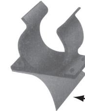
Underneath, it has a sticky pad in place which can be used to provide a good fixing to any flat surface and 4x 2.5mm holes to provide a means for physical fixing if required.
